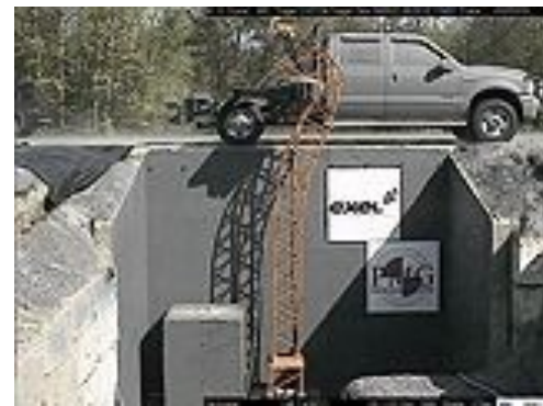
DYNAMIC IMPACT OF LATTICE MAST
